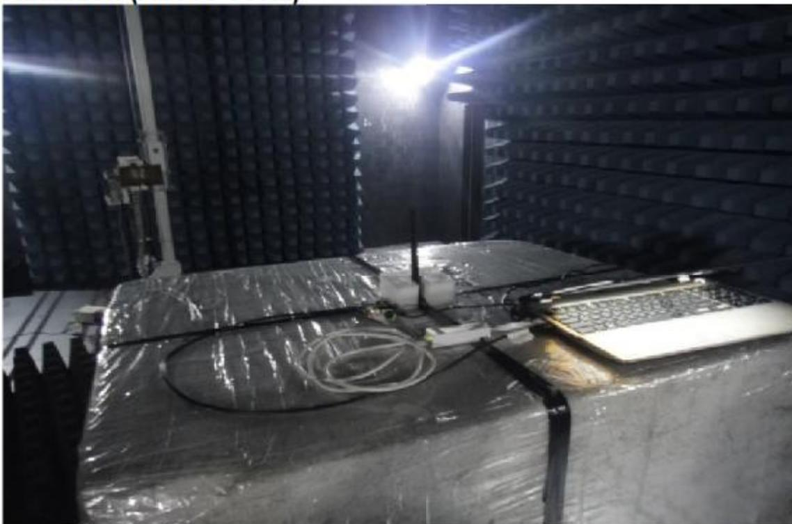
**Conducted Emission Set up Photo**
